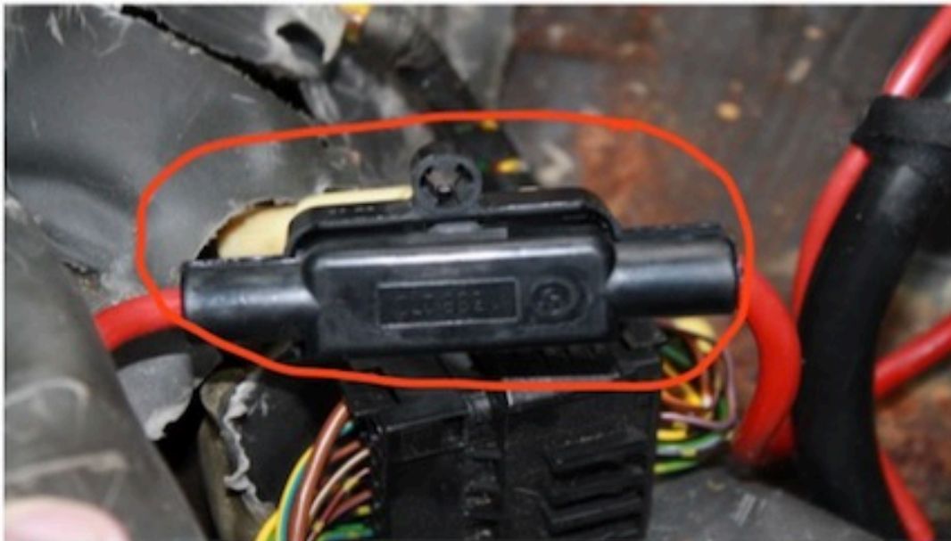
Fusible Link B with cover closed. Just squeeze the cover to open.
