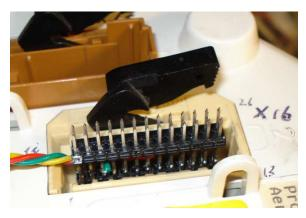
Next re-attach the original X16 connector on top of the piggyback connector.
