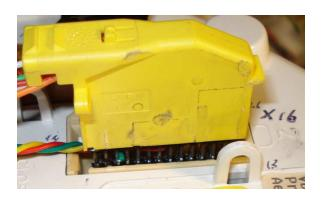
The Piggyback connector DOES NOT provide a proper ground, you must still properly ground pin 1 of the DB9 connector.
