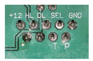
It is very important to properly ground the circuit board. The sensors used rely on the car frame for the return signal to the board. This means that each sensor has a single wire going to the board and the car frame forms the return line for the signal. You will have to verify that the sensors are properly grounded. Not all engine parts, such as remote oil filters are properly grounded. Improperly grounded sensors will cause incorrect readings.
