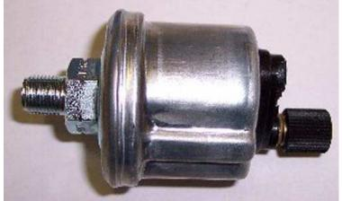
2 wire sensors need to have 1 wire connected to either the car frame <u>or</u> run back all the way to the interface, DO NOT DO BOTH!
