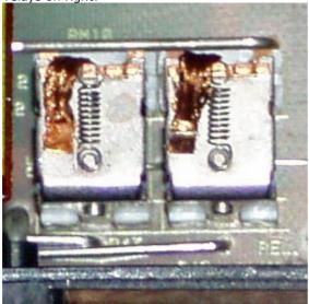
I have heard reports of limited success by just softening the existing solder and letting it harden, but I recommend replacing the solder for all 3 (or 4) relays.
